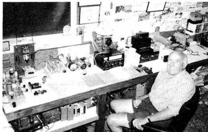
Bill Barnes, ZL2OD, who was licensed in 1933, in his station at Masterton. Bill's transmitter for 14MHz is homebrew with an RK20 final, and his receiver is a rare Drake 2B. He uses an end-fed Zepp antenna
