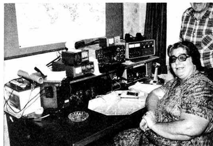
The station of Pauline Carr, ZL2QW, of Featherstone, North Island. Pauline, who makes herself heard worldwide, runs an FT101Z and a seldom-used 2100B linear. The main antenna is a Yagi TH3 Hi-Gain Mk3, with a dipole for lower frequencies
